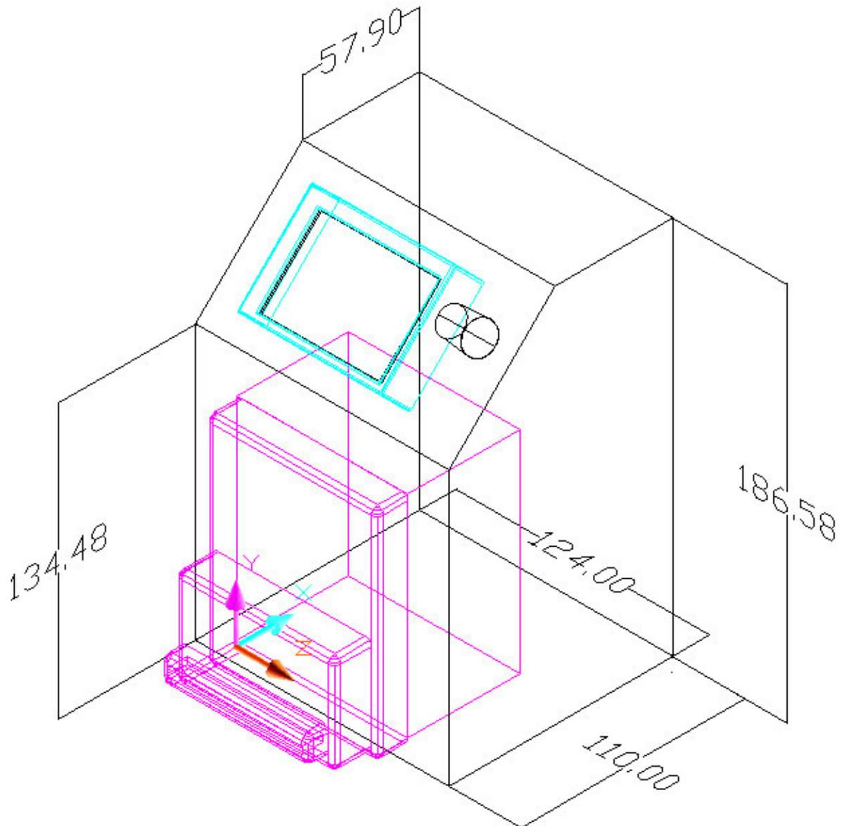
Figure 5 – Control Unit 3D View
