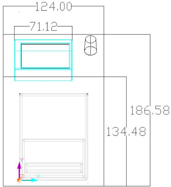
Figure 7 – Controller Front View
